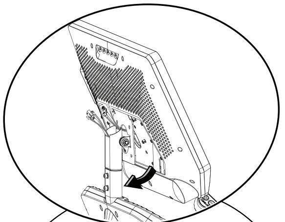
a. Place the Console onto the Console Mast and route the Cables through and out of the Console Mast
