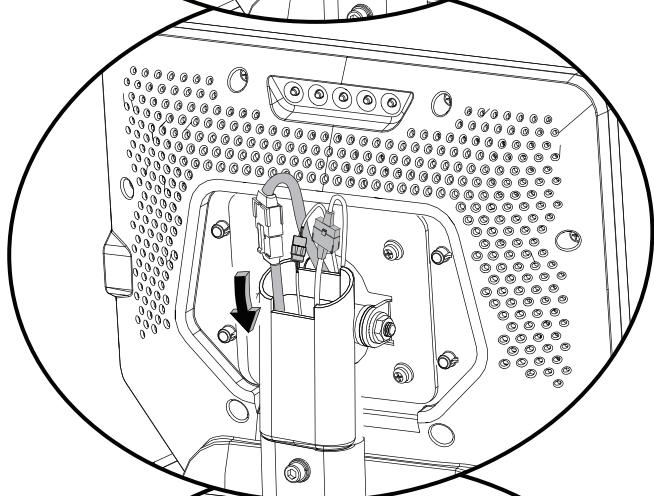
d. Gently slide each of the Connectors and their Cables down into the Console Mast in the following order:
