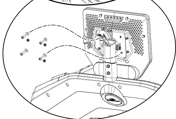
b. Fully pivot the Console Assembly downward and secure it to the Console Mast.
