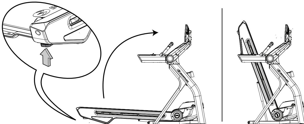
**!** Do not use the walking belt or rear roller to lift the treadmill. These parts do not lock in place and can abruptly move. Injury to you or damage to the machine can occur.
