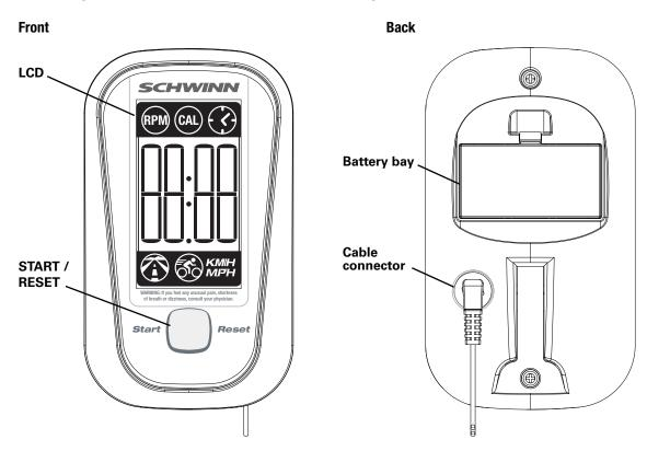
START/RESET Push to start, or to stop an active workout and reset the Time to 0:00.
