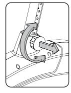
Loosen and pull the adjustment knob on the seat tube. Adjust the seat to the desired height. Release the adjustment knob to engage the locking pin. Be sure that the pin is fully engaged and fully tighten the knob.
