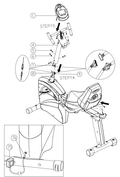
Assembly Hardware Required: (4) Allen Bolts 16 mm long (item #5) (4) Curved Washers (item #6) (4) Computer Screws (item #3)
